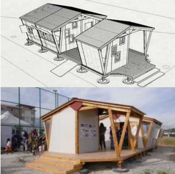
Images: Timber construction technique (HiM, 2023)
